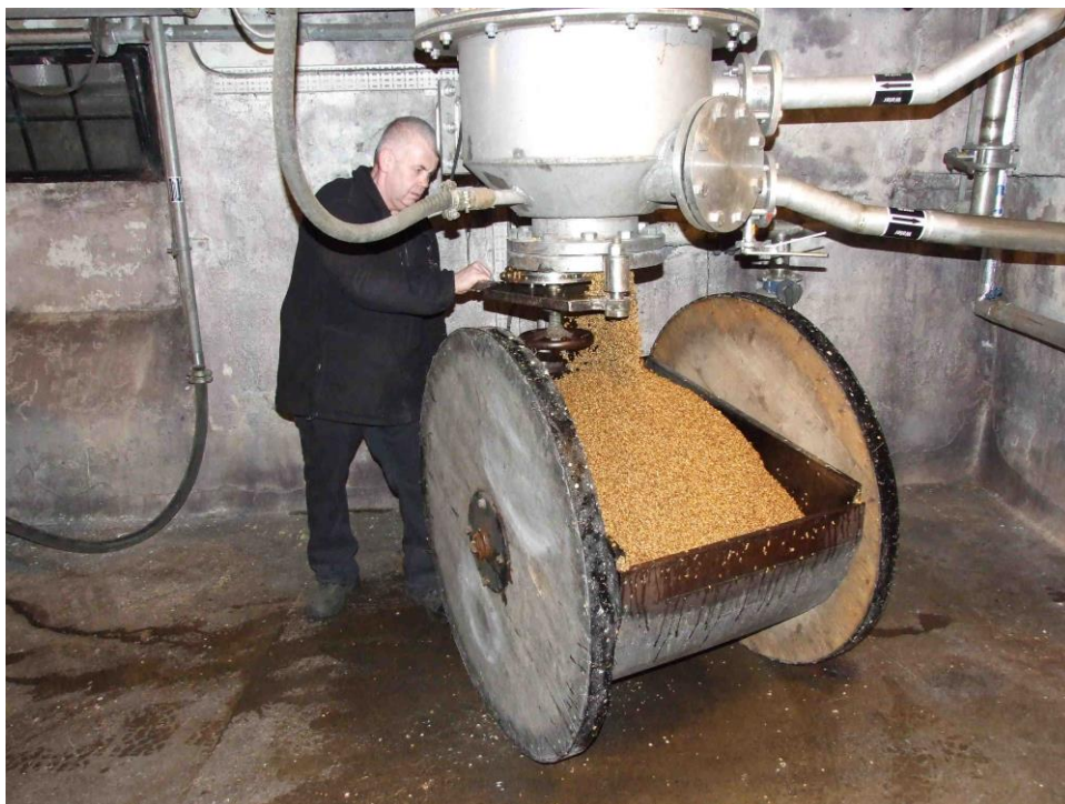
Photo 5. Unloading grain from the steeping vessel.
