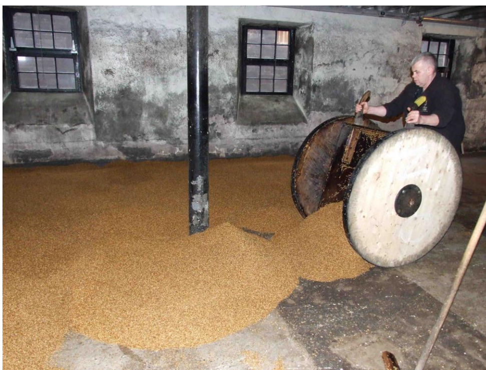
Photo 6. Casting steeped grain on the malting floor.
