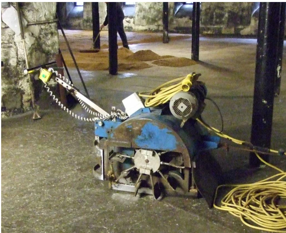
Photo 8. Machine used for turning malt
