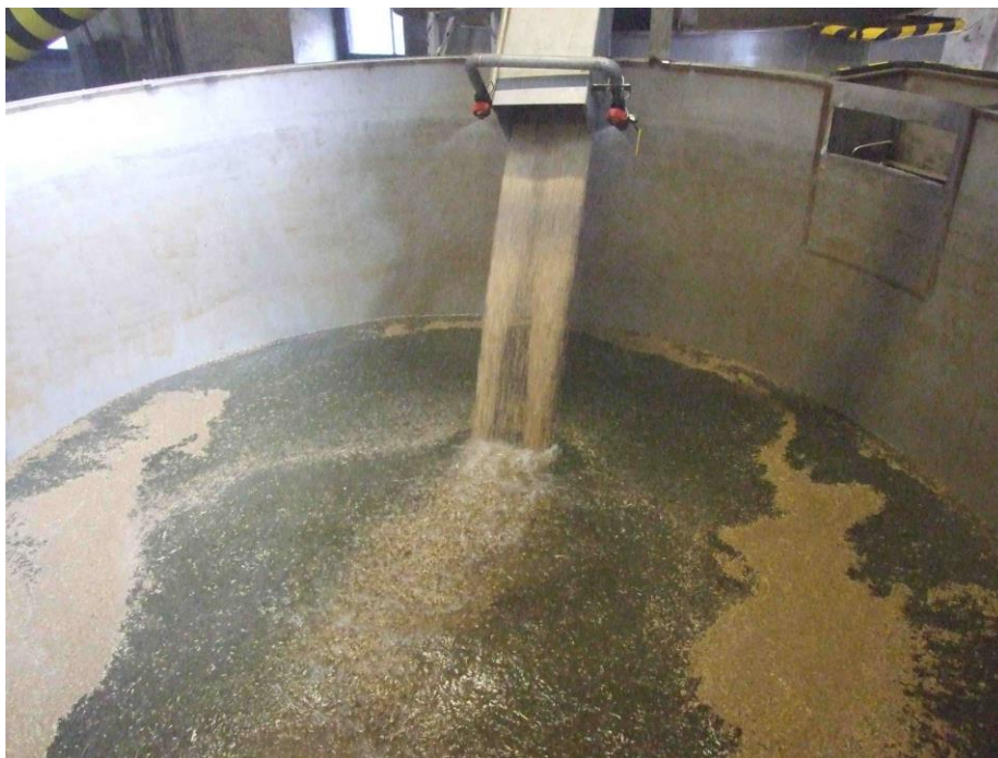
Photo 1. Transferring grain into the steeping vessel.
