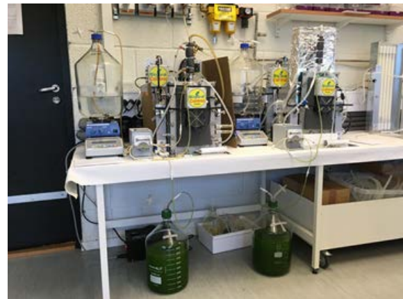
Figure 3. Set-up of photobioreactor
