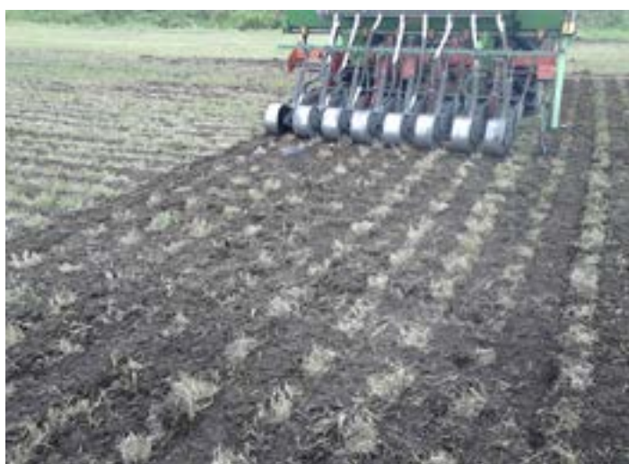
Cross-under-sowing with a rotary band-tilling seeder with tine cultivator (cutter). Photo: J. Barszczewski.
