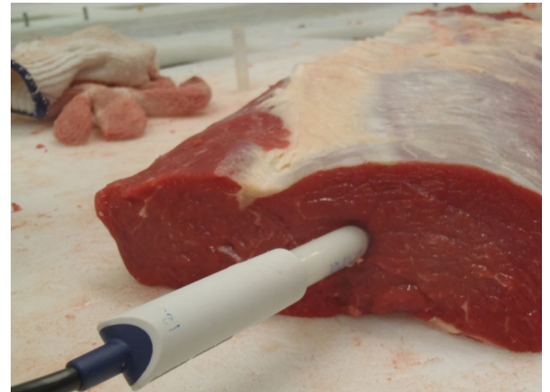
Measurement of ultimate pH 24hours in meat from the loin muscle (M. longissimus dorsi). Photo: Karin Wallin
