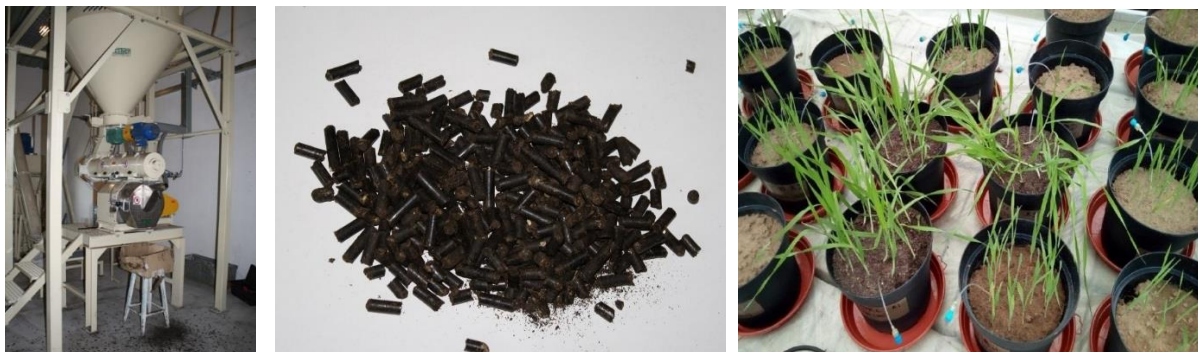
Fig. 3. Production of compost pellets by the SGGW partner and pot experiment carried out by INRA © Wieslaw Szulc, Rafael Gomez
