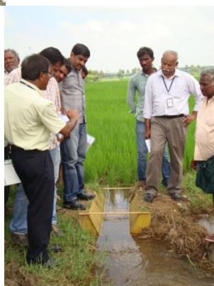
Poorly functioning RBC flume with no difference in water level
