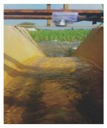
RBC flumes and flow meters were installed to accurately measure the water flow in the field channels. The water depth in the field was monitored with the help of Bowmen tube. Ultrasonic sensors were used for accurate measurement of water depth, both in the flume and in the field. This has helped in educating the men and women farmers, field
